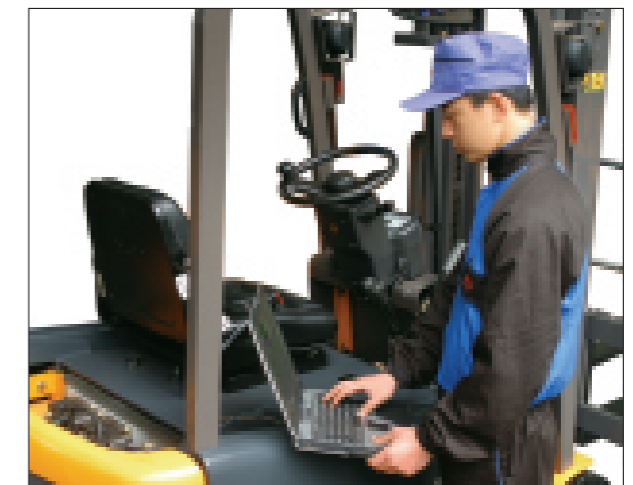
More than thirty performance parameters can be adjusted to suit the type of load, congestion of the working area and skill of the driver.
